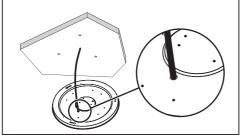
6. Fix the pan on the ceiling with screws.
