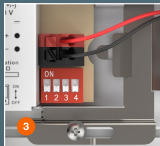
DIP switch for easy power steps setting.
