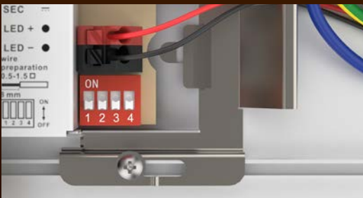
DIP switch for easy power steps setting
