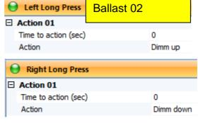
Disable Shortpress, Longpress, Doublepress for the button 'Top' to avoid unwanted activation during wheel turn by the button in the middle.
