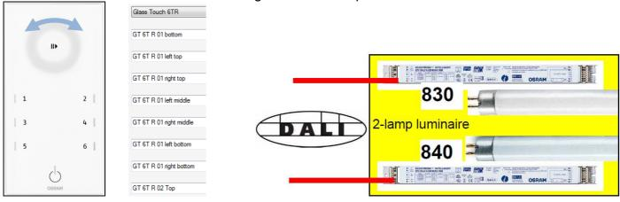
Configure 'Left Long press' to Dimm down and 'Right Long Press' to Dimm up for one ECG and 'Left Long press' to Dimm up and 'Right Long Press' to Dimm down for the other
