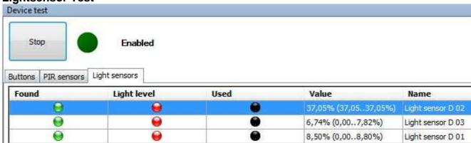
Value changes >20% result in green level dot when sensor reacted on change (e.g. light torch / shadow)
