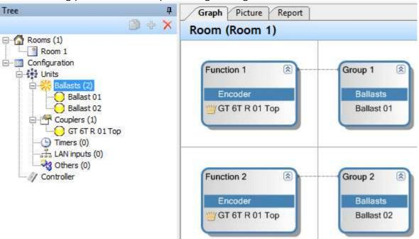
The crown occurs as reminder because same input device button is used in different functions
