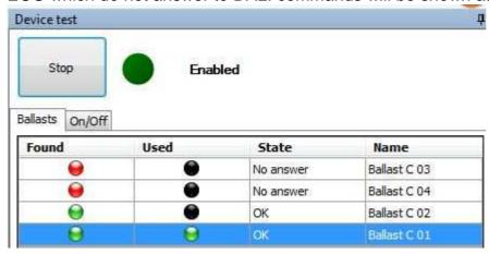
ECG connected to a failed lamp will be shown with red dot
