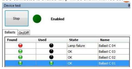
ECG which temporary lost connection to mains voltage will be found Power failure message is shown even after recover until next light change (e.g. ON/OFF)
