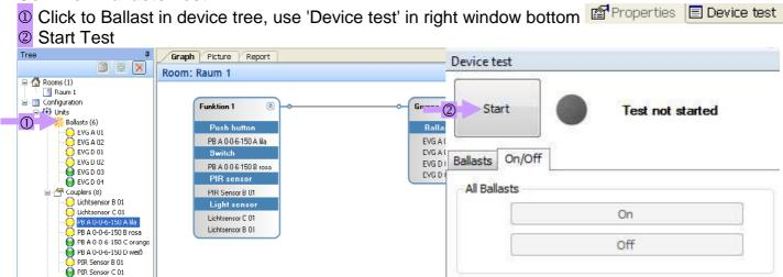
Now all ballast can be switched ON / OFF to localize non reacting luminaires
