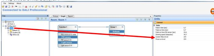
To use the general settings for a individual ballast the "System failure level mode" or the "Power on level mode" has to be set to "General setting". If set to "Individual setting" a ballast specific value can be set.
