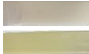
Difference between an OSRAM LINEARlight FLEX® DIFFUSE and another LED strip with evident yellowing effect
