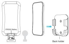
**Note:** Please install the 3V 2032 battery cell first inside the battery case at the back side before using the remote controller.
